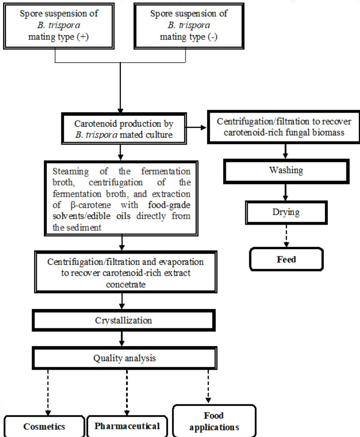
Figure 6. Flow diagram of production of carotenoids by *B. trispora*<sup>18</sup>.
